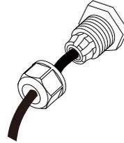
3. Remove the cable jacket and strip the wire insulation.
