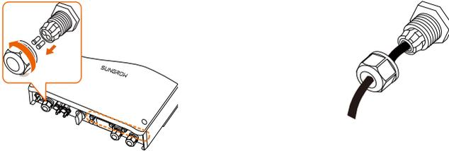
3. Remove the cable jacket by 40 mm to 50 mm and strip the wire insulation by 5 mm–7 mm.
