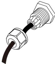
3. Lead the cable through the cable gland, as shown below.
